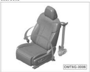
In the event of a vehicle collision, the seat belt, if fastened correctly, can restrain the driver and passengers in a proper position and slow down the inertia of their forward movement, thus preventing them from being thrown forward, and at the same time allow airbags to give them the best protection, thus reducing their impact injury as much as possible.
