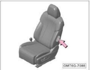
Front seat side airbags are installed at the outboard side of the driver's seat back and that of the front passenger's seat back (as indicated by the dotted dash) marked with "AIRBAG".
