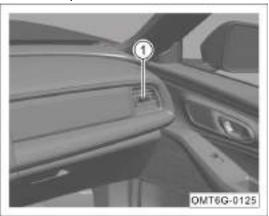
Move the vent control tab ① to adjust the airflow direction or to close the air outlet.
