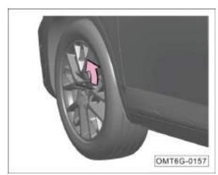
Set the wheel bolt removal wrench firmly on the wheel bolt, and unscrew the wheel bolts counterclockwise.
