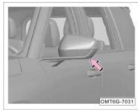
The left/right camera is installed on the left/right exterior rearview mirror respectively.
