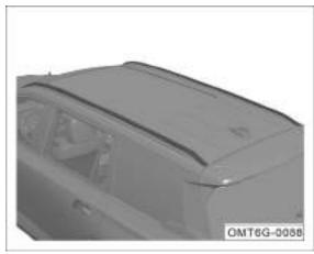
Roof rack of this vehicle can carry a maximum of 50kg of items and overloading is prohibited.
