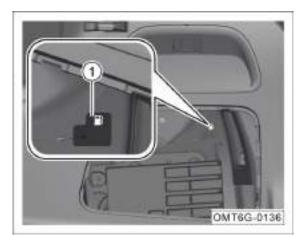
2. Pull the emergency cable ① to open the fuel tank cap.
