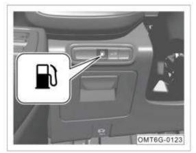
Press and hold the fuel tank cover opening button and fuel tank flap will pop up.
