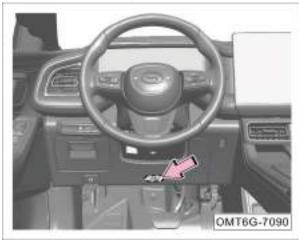
The driver's knee airbag is installed inside the instrument panel (as indicated by the dotted dash) marked with "AIRBAG".
