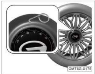
1. For models with floating wheel markers, disassemble the covers of the floating wheel markers before disassembling wheels. Use a floating wheel maker disassemble tool to pry open the cover from the small hole.
