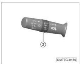
When the vehicle power is in the "ON" gear and position lamp or low beam are on, rotate fog lamp ② to turn on or off  $\{0\}$  (front fog lamp) and  $\{0\}$  (rear fog lamp).
