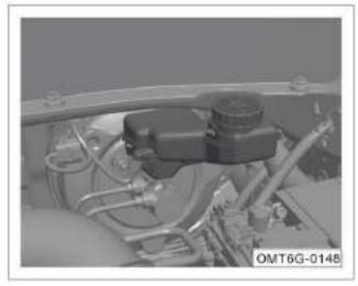
When the engine cools down, check whether the brake fluid level is between the upper limit mark "MAX" and the lower limit mark "MIN".
