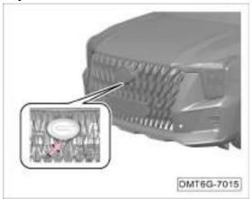
The front camera is installed under the front logo.
