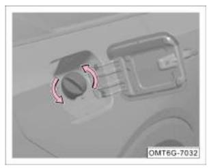
2. Open the fuel tank flap completely, and slowly unscrew the fuel filler cap counterclockwise as arrowed. Keep the fuel filler cap at the original place for a while before it is unscrewed completely to allow the fuel tank to release the fuel vapor inside, and then remove it.
