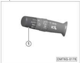
When the vehicle power is in the "ON" gear, rotate the light switch ① to control the AUTO (automatic headlamp), ⇒ (position lamp), or © (low beam).
