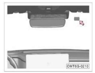
The microwave window is set to the right of the front windshield corresponding to the interior rearview mirror in the vehicle.
