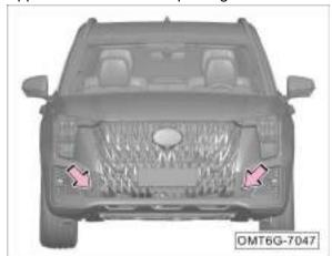
The front ultrasonic sensors are mounted on the front bumper.
