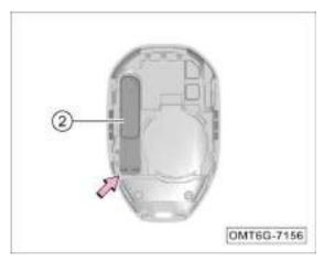
2. Remove the emergency mechanical key ② from the position indicated by the arrow.
