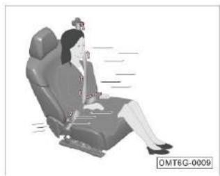
The seat belt pretensioner and load limiter can reduce the pressure of the seat belt on the chest of the driver and passengers and improve the protection performance.
