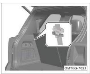
When fastening the 2nd row seat belt/rear seat belt, pull out the clip from the holder in the trim panel before moving out the webbing to slide out of the holder, and then pulling the seat belt for fastening, so as to avoid damaging the holder when pulling the seat belt.
