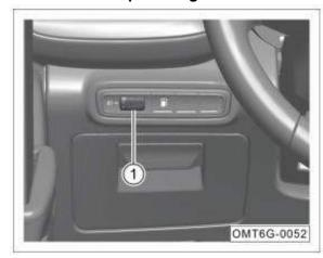
Rotate the knob ① to manually level the headlamp (low beam) at 0, 1, 2 and 3 positions. The level of the headlamp will decrease as the adjustment value increases.
