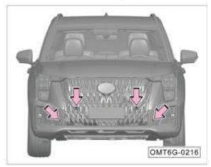
The front ultrasonic radar sensors are mounted on the front bumper cover.
