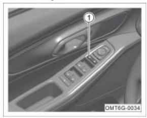
The central locking button ① can lock and unlock the doors inside the vehicle:
