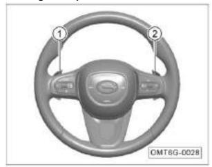
When the vehicle is driving normally, the driver can shift up or down by turning the shift paddles on the steering wheel:
