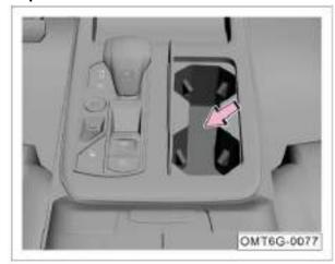
Front cup holder: Press the front cup holder cover to open it and use the cup holder for placing beverage bottles.
