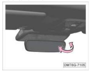
The automatic anti-glare interior rearview mirror monitors the intensity of lights behind the vehicle in real time, and automatically adjusts the reflective effect, so that strong lights it reflects to the driver's eyes turn dark and not glaring.
