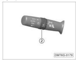
When the vehicle power is in the "ON" gear and position lamp or low beam are on, rotate fog lamp switch ② to turn on or off Off (rear fog lamp).
