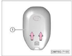
1. Push the back cover ① firmly in the direction of the arrow. After hearing a "click," remove the back cover ①.
