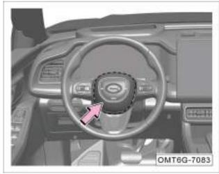
The driver's frontal airbag is installed inside the steering wheel (the shaded area) marked with "AIRBAG".
