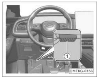
The OBD interface ① for reading the electronic VIN is located on the lower left side of the instrument panel, and can be used with a diagnostic scan tool to read the electronic VIN and vehicle information.
