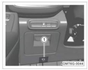
Pull engine compartment ① under driver's side instrument panel twice. Engine compartment will pop up slightly to a fully unlocked state. Now you can open engine compartment outside the vehicle.
