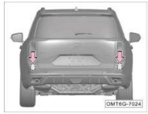
The BSD radar sensors are installed as shown above.
