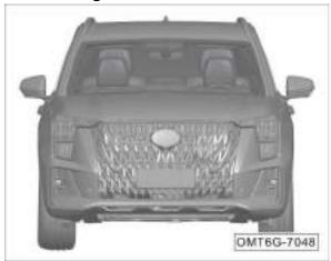
The front windshield is made of green soundinsulating and laminated anti-scattering glass, which can effectively reduce the degree of accident injuries.
