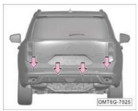
The rear ultrasonic sensors are mounted on the rear bumper.
