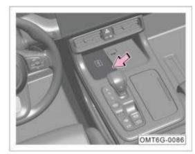
The effective wireless charging area is located in the storage compartment in front of the gearshift lever. During charging, align the phone's charging coil with the "Qi" symbol to ensure proper charging.
