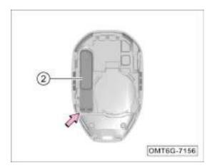
2. Pick up emergency mechanical key ② in the direction of the arrow.
