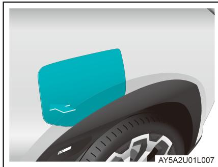
1. Unlock the vehicle, and press the rear edge of the charging inlet cap to open it.
