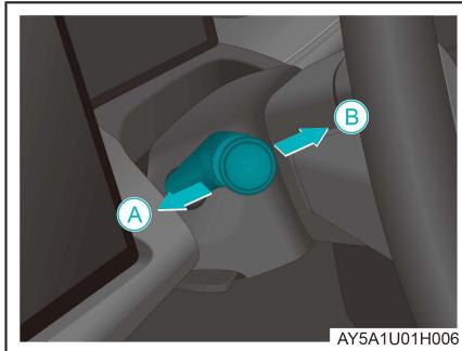
After the headlamp is on, push the light/wiper control lever in the direction of arrow A to switch the headlamp to the high beam, and pull back the light/wiper control lever in the direction of arrow B to turn off the high beam.
