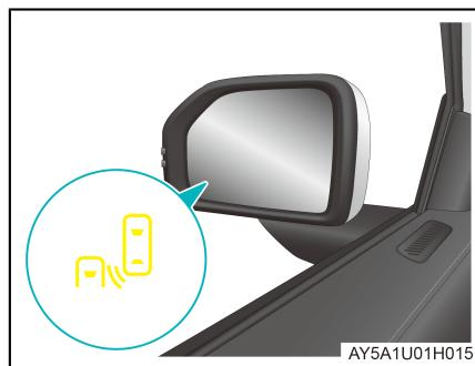
During reversing, if the system detects a vehicle approaching rapidly from the side or rear, the warning lamp on the corresponding side exterior rearview mirror will flash, accompanied by an audible alert. The instrument panel will also show a red warning symbol for the rear danger zone, indicating that continuing to reverse may be dangerous.
