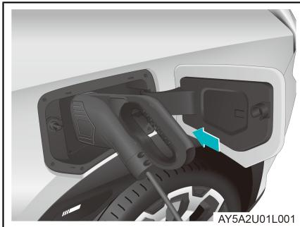
3. Insert the charger as arrowed. After the charger is successfully connected, all turn signal lamps will become yellow and on for a long time, and the charger indicator lamp
