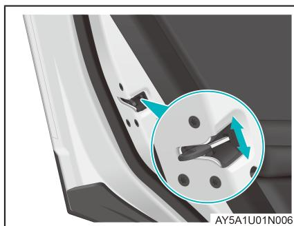
2. Insert the mechanical key into the keyhole in the door lock, turn the key downward to the locked position, pull out the mechanical key, and close the door to lock the door.
