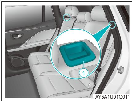
2. Pull the folding handles ① on the left and right of rear seat to unlock the rear seat back.
