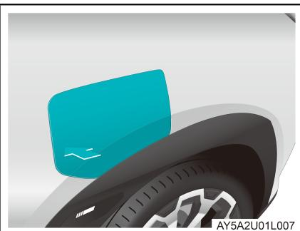
1. After the vehicle is unlocked, press the rear edge of the charging inlet cap to open the charging inlet cap.
