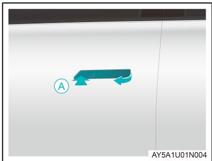
1. Unlock the vehicle, and push the front side of the handle (arrow A) to turn the other side up.
