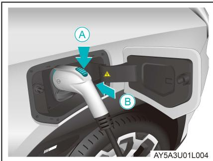
3. While pressing the charger button in the direction of arrow A, insert the charger in the direction of arrow B. After the charger is successfully connected, all turn signal lamps become yellow and on for a long time, and the charger indicator lamp
