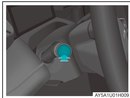
Press the front wiper washer button to have the front washer nozzle spray washer fluid. After the wiper control lever is released, the front washer nozzle stops spraying the washer fluid, the wiper operates several times, and then operates once after a period of time and stops.
