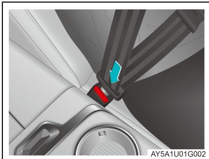
2. Gently pull out the seat belt, route it across the chest and hip, and insert the tongue into the buckle until you hear and feel the latch engage.
