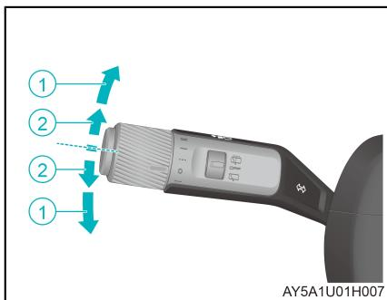
Turn signal: Move the light/wiper control lever to ① position. After you release it, the light/wiper control lever will automatically return and the corresponding side turn signal lamp will flash continuously. After the steering wheel returns, the turn signal lamp will turn off automatically.
