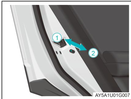
When a child takes a rear seat, please move the switch to locking position ② before closing the door. At this time, the door cannot be opened from inside, so as to prevent the child from opening the door unexpectedly.
