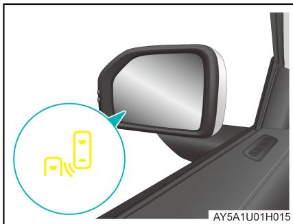
If a vehicle or pedestrian approaches the vehicle while parked, the corresponding side exterior rearview mirror warning lamp will light up, prompting the driver and passengers to check the safety of the environment before opening the door. If the door on the alerted side is opened, the exterior rearview mirror warning lamp will start flashing, and the system will emit an audible alert, indicating that continuing to open the door may be dangerous.
