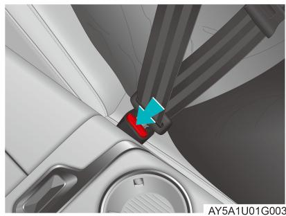
1. Hold the seat belt and press the red button next to the seat belt buckle, so the tongue will spring up automatically.
