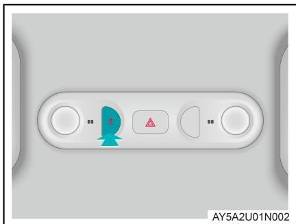
When the vehicle is powered on or in motion, pressing the emergency power off switch will prompt a related message on the instrument panel. At this time, holding the emergency power off switch for a period or pressing the switch three times in quick succession will initiate an emergency power off.
