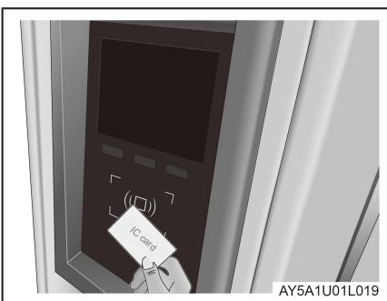
4. Make relevant settings on the charging pile (such as scanning QR code or swiping a card), and start the charging pile.
