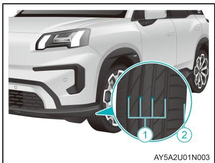
There is a raised "tread wear indicator" ① on the front of the tire. If the tread pattern wears to the indicator surface, the tire can no longer be used safely and must be replaced immediately.
