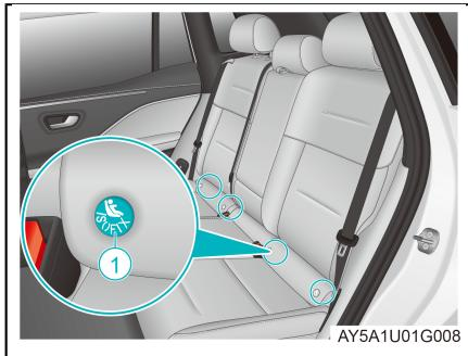
There are four ISOFIX/ISIZE anchorage provided between the rear seat back and the rear seat cushion for installation of child seat. Label ① is used to indicate the position of ISOFIX/ISIZE anchorage.
