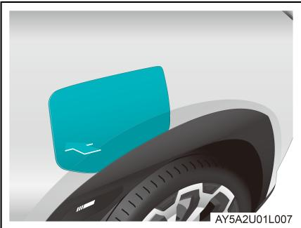
1. Unlock the vehicle, press the rear edge of the charging inlet cap to open it.
