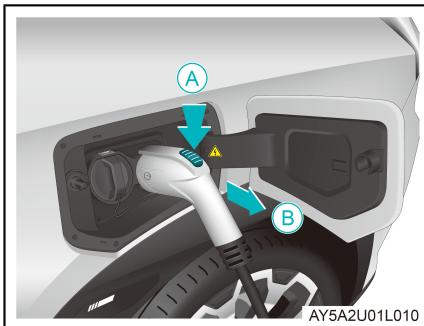
7. Unplug the charger in the direction of arrow B, while pressing the charger button in the direction of arrow A.
