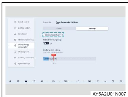
4. Enable the discharging function by tapping on the discharging soft key on the center console display within 140s. The red indicator lamp of the discharging power strip will be turned on. Please connect the electrical consumer.
