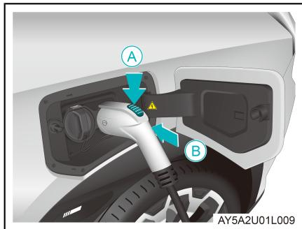
3. Insert the discharger in the direction of arrow B, while pressing the discharger button in the direction of arrow A.
