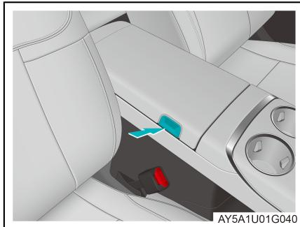
Press the vehicle refrigerator lid's open button to lift the lid and access the refrigerator.
