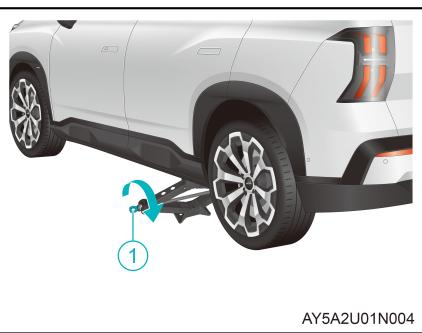
2. Turn the jack ① clockwise so that the jack is close to the lifting point of the body.
