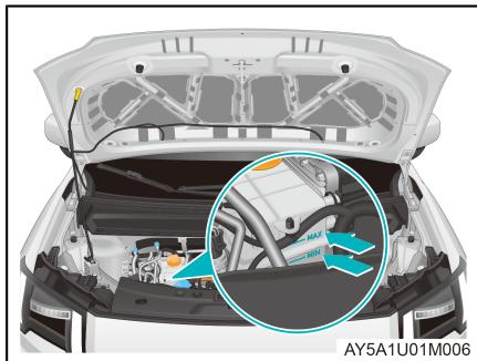
Open the hood, and check the coolant level in the expansion tank. If it is below the "MIN" mark, please fill the expansion tank with coolant to the level between the "MIN" and "MAX" marks in time.
