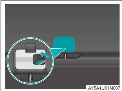
2. Remove the liftgate emergency unlocking port cover from the liftgate guard plate. Toggle the unlocking switch in the direction of the arrow as shown to unlock the liftgate.
