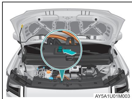
1. Hold the hood by hand, and take away the stay bar to fix it to the position as shown in the figure.
