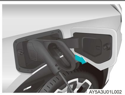
7. Pull out the charger as arrowed.
