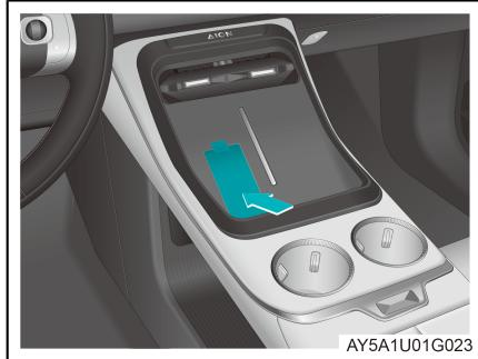
Place a mobile supporting wireless charging in the wireless charging area. To ensure good wireless charging experience, it is suggested the mobile should be close to the rear air outlet of the charging area, and align the mobile charging coil with the charging area shown in the image.
