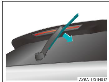
2. Pull out the wiper blade in the direction of the arrow to remove it.
