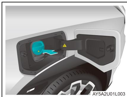
2. Open the dust cover of the AC charging inlet.
