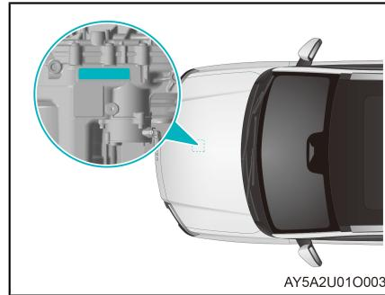
The motor model and number are engraved on the motor housing.
