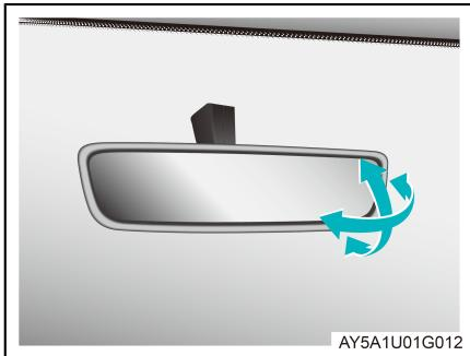
Adjust the interior rearview mirror up and down, left and right to the best rear view position.
