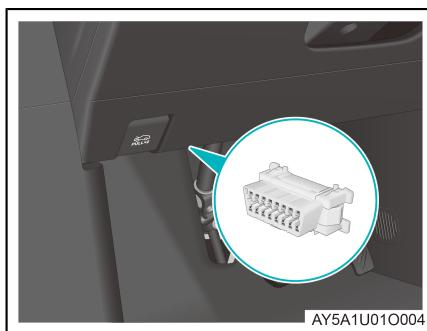
The OBD DLC is located at the lower right rear of the instrument panel. Data such as the vehicle identification number (VIN) and vehicle status information can be read by connecting a special diagnostic scan tool to the OBD DLC.
