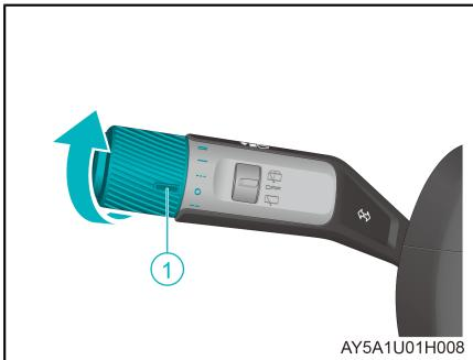
Turn the wiper control knob up or down from the O position, so that the front wiper position icons are aligned with the wiper control knob position reference icons ① in turn, and the front wiper mode can be selected. The specific control is as follows:
