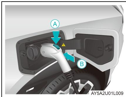
3. Insert the charger in the direction of arrow B, while pressing the charger button in the direction of arrow A. All turn signal lamps turn on for quite a bit of time when the charger is correctly connected, and the instrument's Charger Connected indicator lamp
