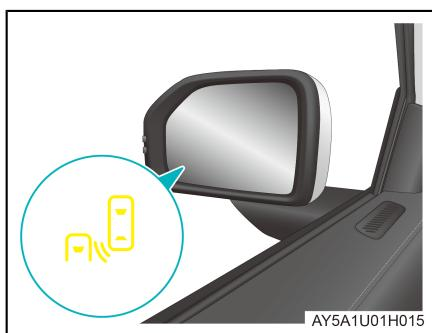
While driving (at speeds greater than 15 km/h), if another vehicle enters the blind spot from behind or the side, or if a vehicle rapidly approaches from an adjacent lane, or if a vehicle enters the blind spot from the front and stays there for a while, the warning lamp on the corresponding exterior rearview mirror will light up.
