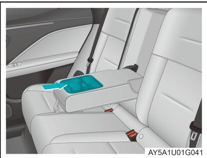
The rear cup holder is in the central armrest. Pull down the armrest before using the rear cup holder.
