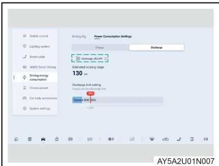
4. Tap the discharging soft key on the center console display within 140 s to turn on the discharging function. The red indicator lamp of the discharging power strip will turn on. Please connect the electrical consumer.
