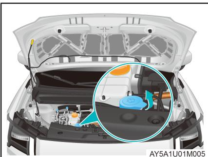
Open the hood, open the washer fluid reservoir cap as arrowed, and check the washer fluid in the reservoir. If the washer fluid level is too low, please add the washer fluid or a mixture of washer fluid and water.
