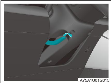
1. Unlock the steering wheel by pulling the steering wheel locking handle down.
