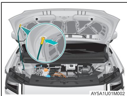
3. Take out the support bar and insert it into the position as shown in the figure to fix the hood.
