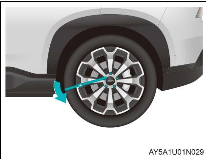
1. Turn the wheel bolts counterclockwise with the wheel bolt wrench, to loosen them by 1~2 turns.
