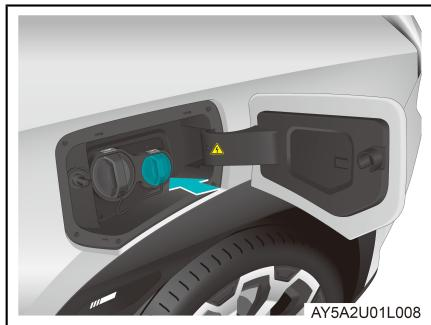
2. Open the dust cover of the AC charging inlet.
