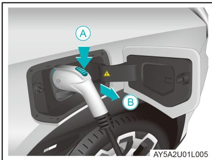
6. After charging, the charger will unlock automatically. While pressing the charger button in the direction of arrow A, unplug the charger in the direction of arrow B.
