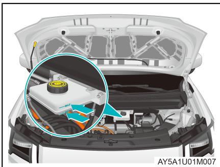
Open the hood, and check the brake fluid level in the brake fluid reservoir. If it is below the "MIN" mark, please fill the brake fluid reservoir with brake fluid to the level between the "MIN" and "MAX" marks in time.
