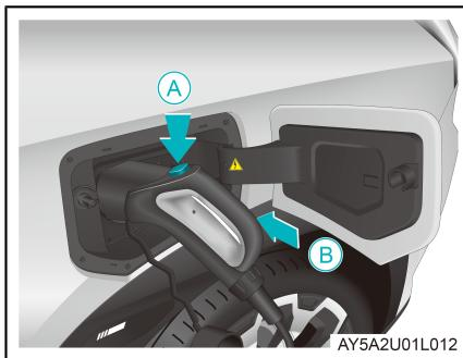
3. Insert the charger in the direction of arrow B, while pressing the charger button in the direction of arrow A. All turn signal lamps turn on for quite a bit of time when the charger is correctly connected, and the instrument's Charger Connected indicator lamp
