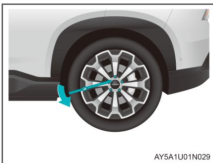
4. Remove the wheel bolts, and take off the damaged wheel.
