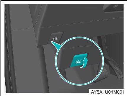
1. Pull up the hood release lever in the cab twice, and then the hood will be unlocked and pop up slightly.
