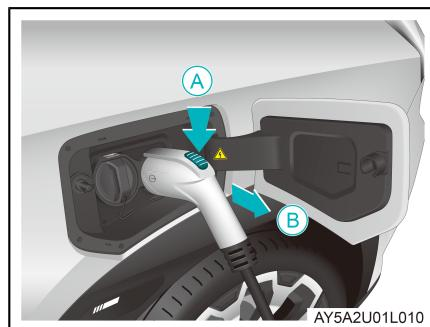
7. Unplug the discharger in the direction of arrow B, while pressing the discharger button in the direction of arrow A.
