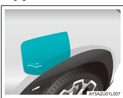
1. After the vehicle is unlocked, press the rear edge of the charging inlet cap to open the charging inlet cap.
