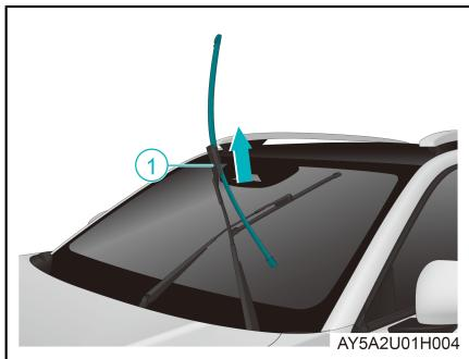
3. Press the wiper blade lock button ①, and remove the wiper blade as arrowed.
